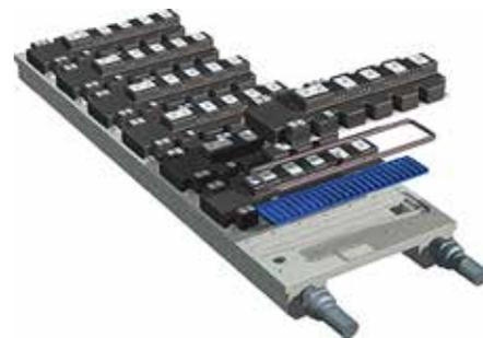
**Die Cast Liquid Cold Plate** is a two piece construction suitable for complex high volume applications. Multiple internal and external features can be incorporated into the two die cast tools. After casting, the two halves can be bonded together by various processes, including welding, brazing or by the use of an epoxy.
