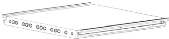
The channels create turbulence, which minimizes the fluid boundary layer and reduces thermal resistance. This also yields excellent thermal uniformity because coolant flows below the entire cold plate surface.
